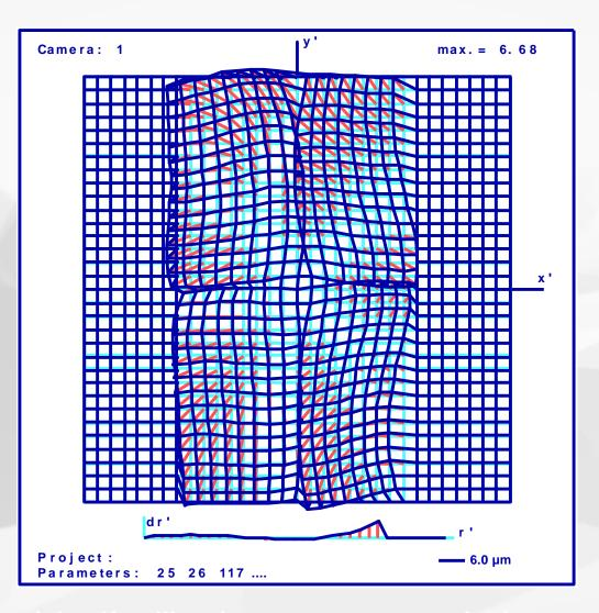
Effects of special self-calibration parameters on the image geometry
