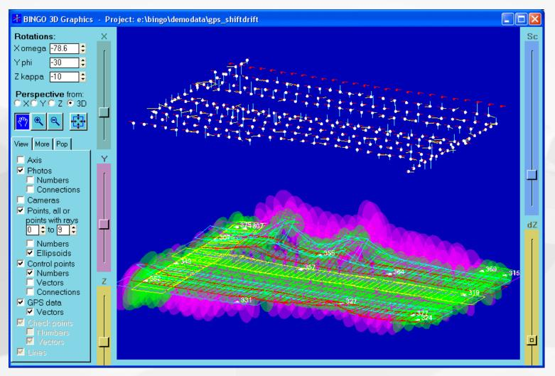
GPS data are missing for the first flight line. As result we have larger confidence ellipsoids in that region.
