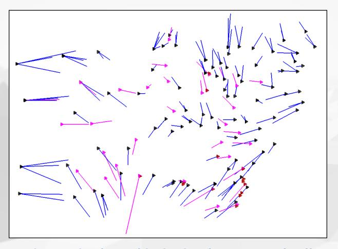
Ground control point residuals showing systematic effects. Additional parameters for different scales in x' and y' remove this problem completely
