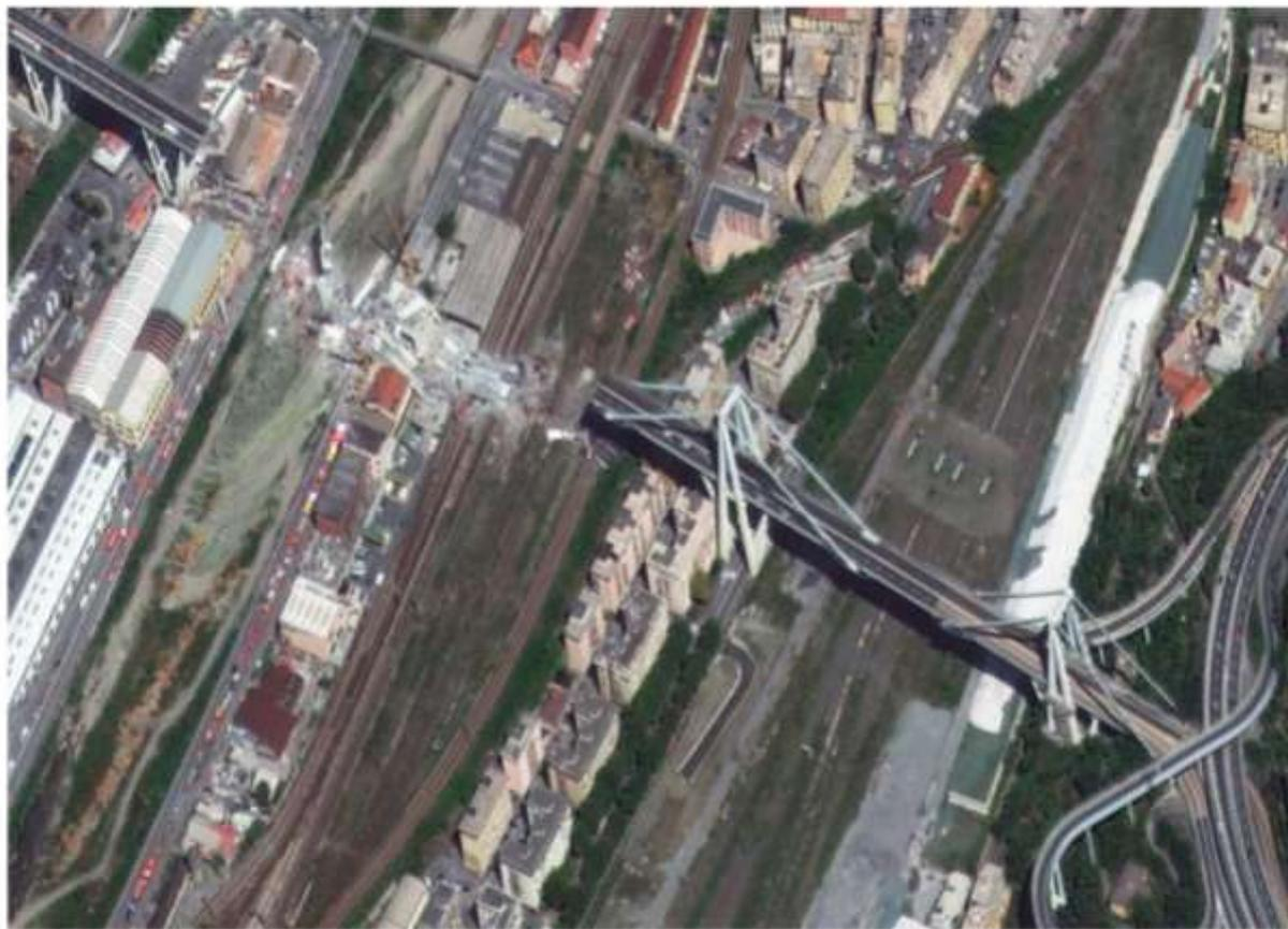
Satellite image at 30 cm resolution showing the collapsed section of Morandi Bridge in Genoa, Italy. The high quality of the data makes it possible to zoom in on the image and thereby identify the extent of the damage. ■ 15/8/2018 by WorldView-4 © European Space Imaging
